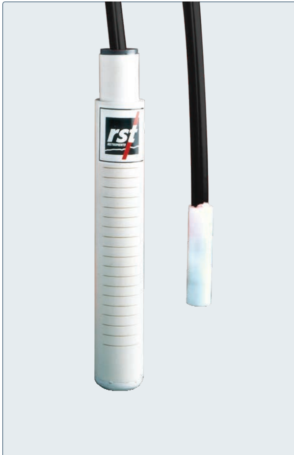
P-100-1 Piezometer (left) and the P-100 Mini Pneumatic Piezoemter
